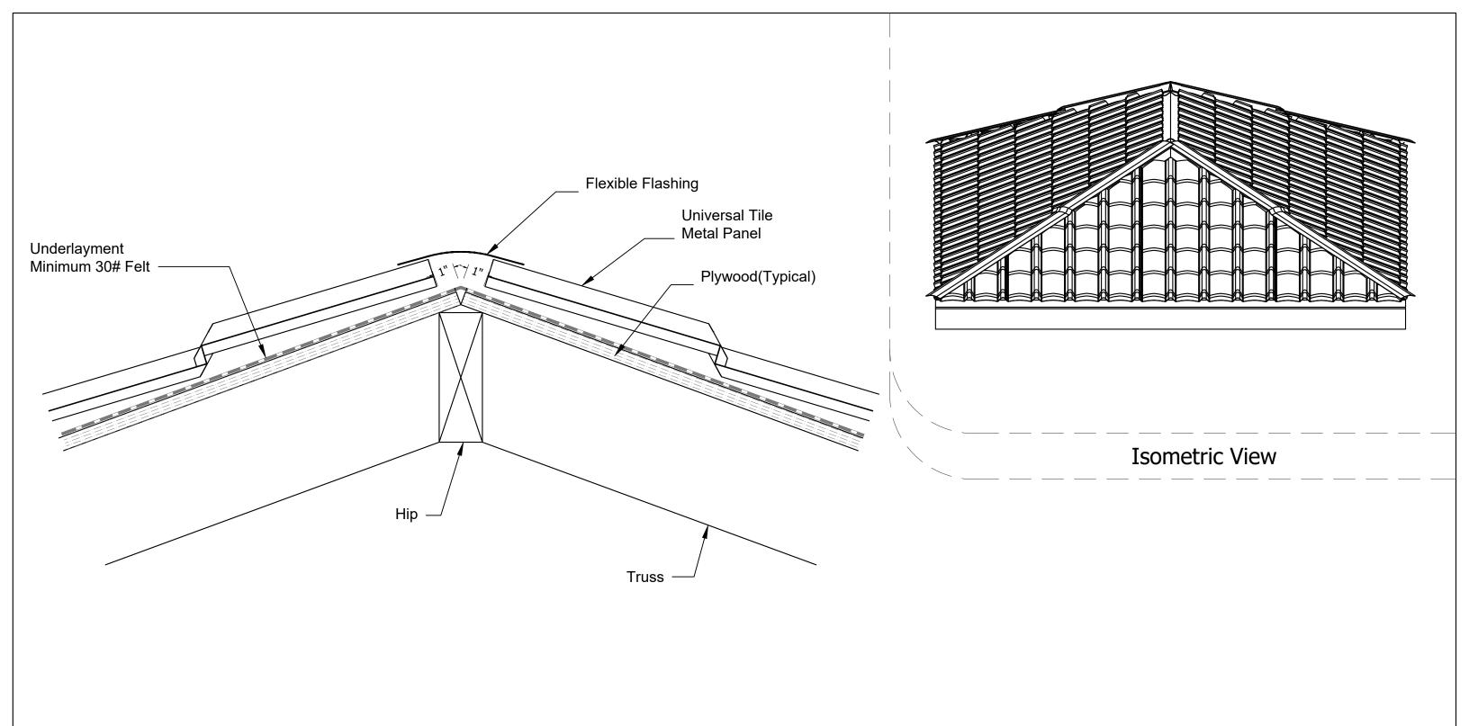
\*Note: Hip Trim Flashing Must Be Installed Before The Flexible Flashing. Flexible Flashing Is installed On Entire Hips And Hip Trim Flashing.
