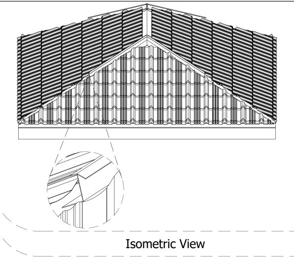
\* Note: Must Install Hip Trim At All Hip To Ridge Connections Hip Trim Flashing Are 4' Long
