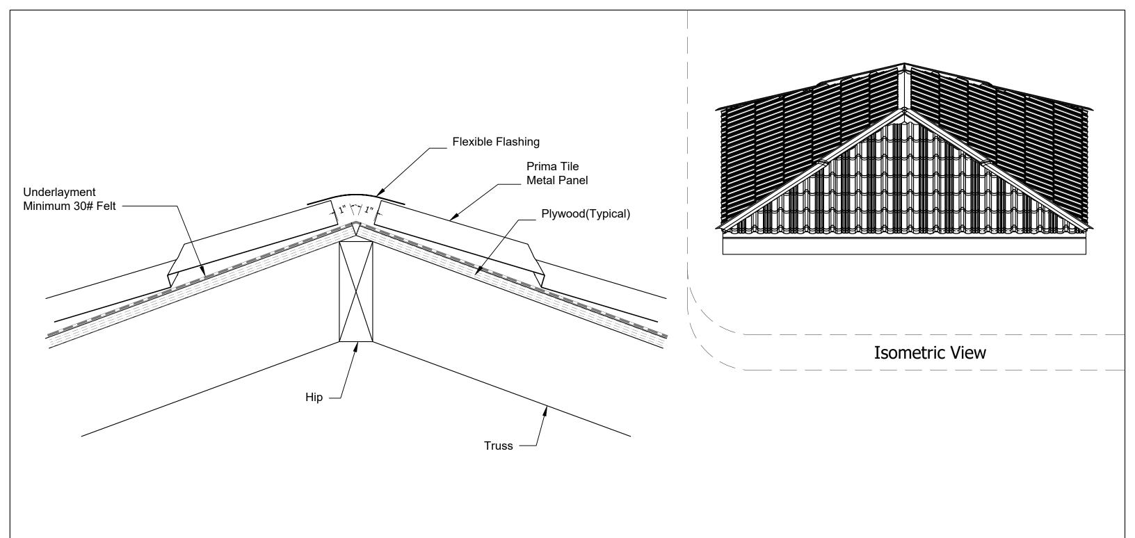
\*Note: Hip Trim Flashing Must Be Installed Before The Flexible Flashing. Flexible Flashing Is installed On Entire Hips And Hip Trim Flashing.
